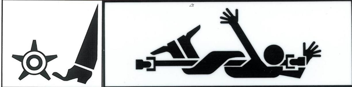
Never use your hands to clear if clogged. Never allow anyone to reach into the rotor housing. The rotor can crush and/or dismember. Keep everyone clear of the rotor until the prime mover engine is off and the hydraulic pressure has been relieved.
